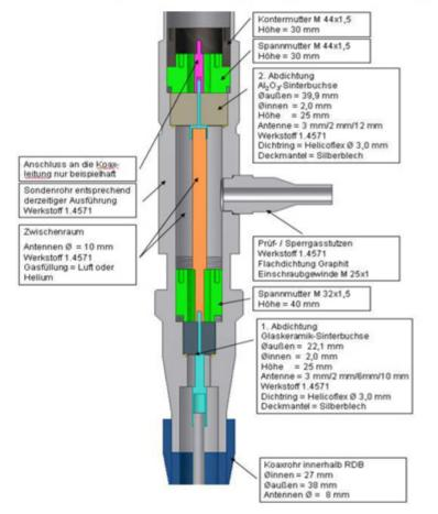
Successful Tests with Prototype Probe Head of AREVA: Level and pressure transients with steam/ deionat up to 170 bar / 350°C
