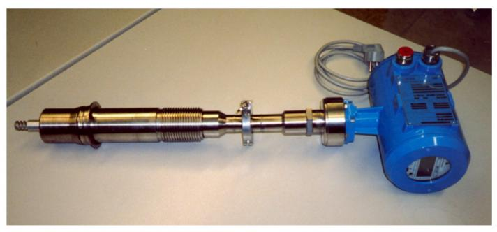
TDR - probe: high pressure probe head for existing RPV nozzle. Layout 230 bar. Probe tube, same diameter like existing Probe (51 mm), easy Backfitting in existing guide tube. Probe length 5 m.
